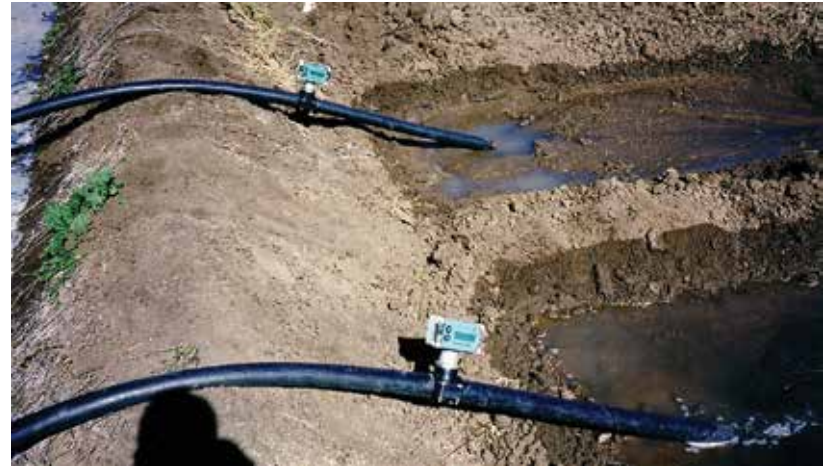
Irrimate Flu Metres (top) and Flow Metres (above) have been used with great success by consultants and growers improve WUE and are a vital tool in quantifying water use – and loss.
