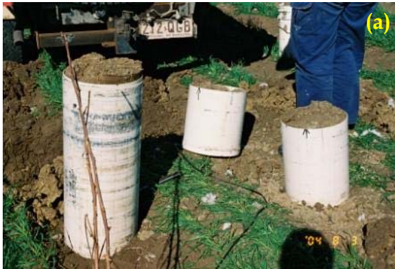
Fig. 3 (a) The three parts of the extracted soil cores. The longer core contains the 0 – 75 cm layer, the two smaller cores contain the 75-105 (right) and the 105-150 cm (center) layer; that becomes the lysimeter. (b) The lysimeter, after plumbing the ceramic candles, silica flour and sealing the base, ready to be lowered back down the hole
