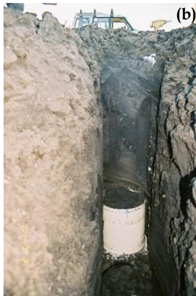
Fig. 4 (a) Lowering the lysimeter back down the hole. (b) The lysimeter in place with plumbed drainage line extending back to the edge of the field (towards the camera). (c), the intact soil cores placed in original order on top of the lysimeter, before the hole and access trench is in
