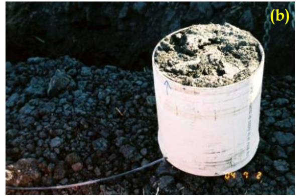
Fig. 3 (a) The three parts of the extracted soil cores. The longer core contains the 0 – 75 cm layer, the two smaller cores contain the 75-105 (right) and the 105-150 cm (center) layer; that becomes the lysimeter. (b) The lysimeter, after plumbing the ceramic candles, silica flour and sealing the base, ready to be lowered back down the hole
