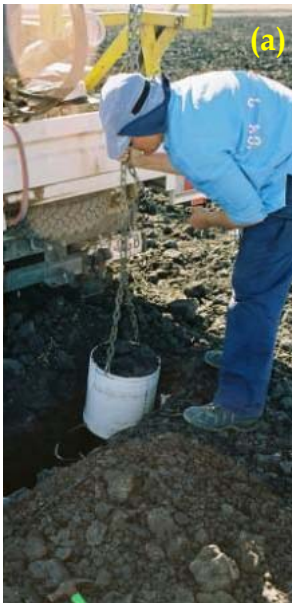
Fig. 4 (a) Lowering the lysimeter back down the hole. (b) The lysimeter in place with plumbed drainage line extending back to the edge of the field (towards the camera). (c), the intact soil cores placed in original order on top of the lysimeter, before the hole and access trench is in
