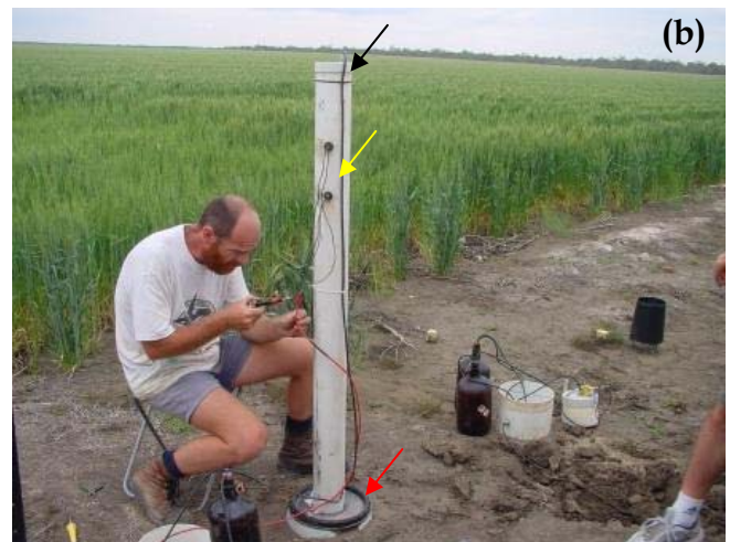
Fig. 5 (a) Building the lysimeter-related apparatus in the field. (b) Plumbing the vacuum tower that supplies the vacuum to the lysimeter. Arrowed are the water reservoir (red), reed switches (yellow) and vacuum supply line (black). The electrical pump (Fig. 6) draws the water up past the lower reed switch, to the upper switch that triggers the pump “off” – creating a vacuum as the water drops back down the column. Passing the lower reed switch, the pump is switched back “on” to again raise the water in the tower.
