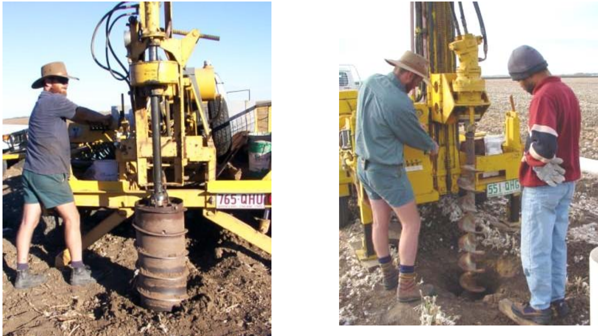
Fig. 1 The proline barrel used to extract intact soil cores of 30 cm diameter (in 2 pieces, encased in plastic “liners”) to 150 cm depth. The deeper of the two cores is split in the middle; the lower part becoming the lysimeter.
