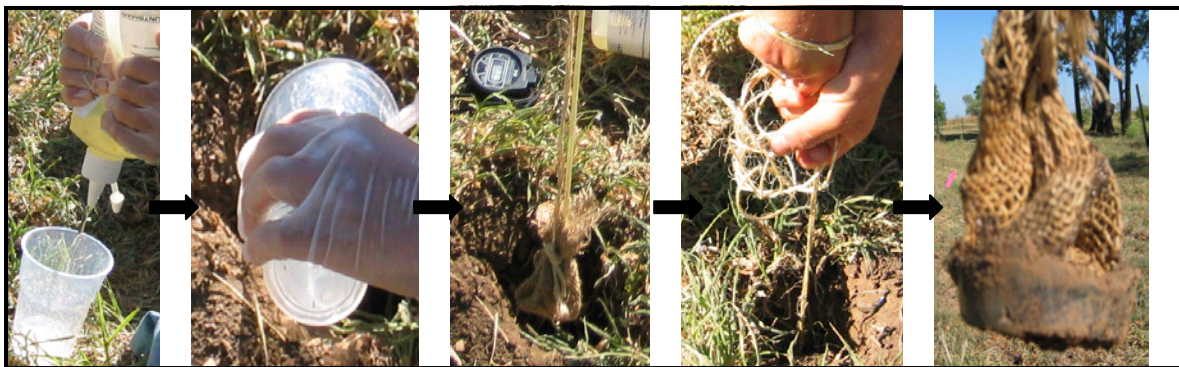
Fig. 19. Treating a hole with araldite using the hessian and twine method
