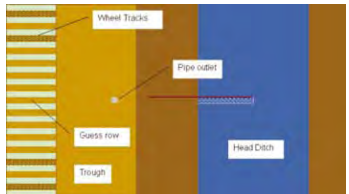
FIGURE 2: erial view of PTB irrigation demonstrating pipe outlet situated in Guess row away from wheel tracks
