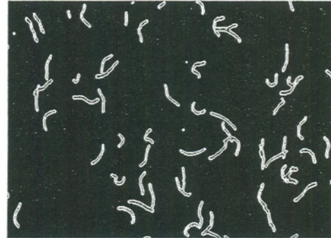
Figure 7 Typical Unprocessed Image Captured by the Cottonscan Instrument
