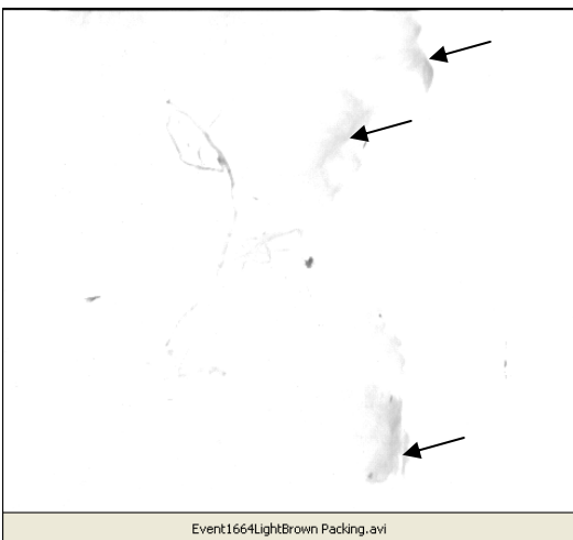
Figure 19 – Light-brown coloured packing material under prototype illumination. Slight shadowing of cotton batt is evident (see arrows)
