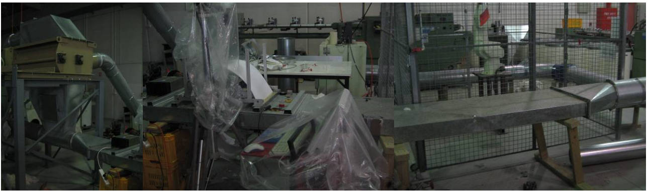
Figure 5 – Re-circulating duct for testing contamination illumination and sensing (a) air separator, exhaust connection and material drop zone, (b) contamination illumination, showing later concave reflecting surface and sensing window, and (c) return duct showing bends after sensing area
