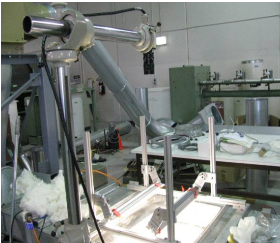
Figure 7 – Viewing window showing camera and initial arrangement of LED arrays to illuminate moving fibre samples
