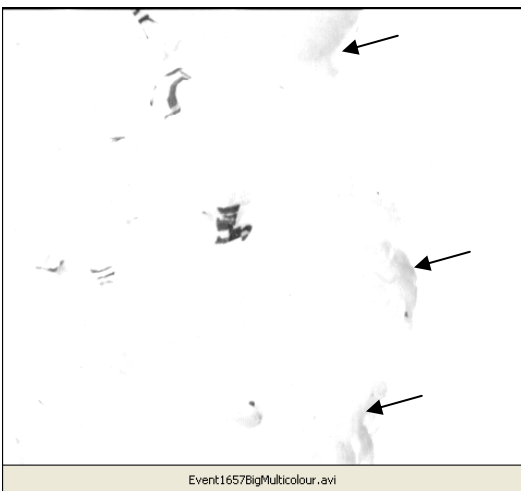
Figure 15 – Multicoloured plastic under prototype illumination. Slight shadowing of cotton batt is evident (see arrows)
