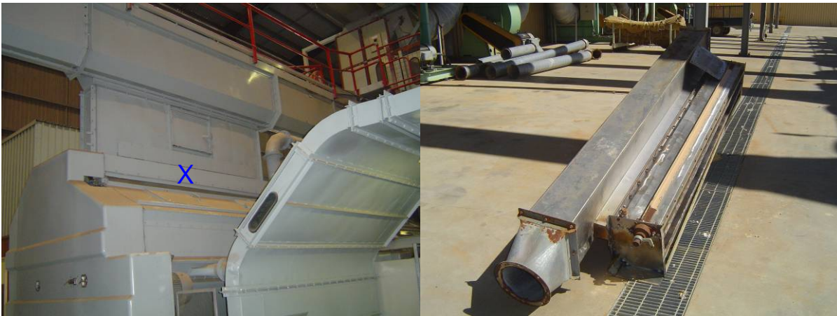
Figure 4 – (a) X marks position of humidifying hopper in gin stand and (b) duct that was fitted to deliver humidified air into cotton before ginning
