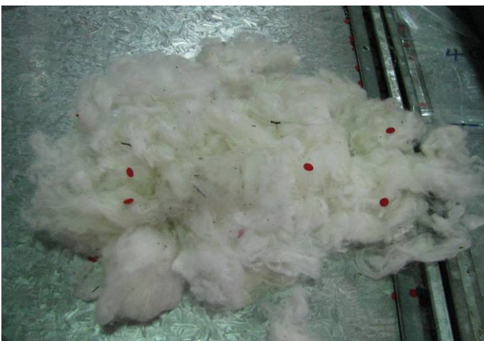
Figure 8 – Cotton spiked with ‘contaminant’ before insertion into the circulating duct
