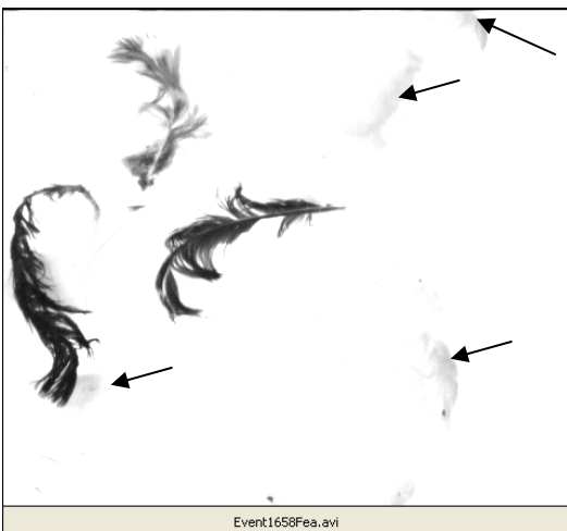
Figure 16 – Feathers of various colours under prototype illumination. Slight shadowing of feathers and cotton batt is evident (see arrows)
