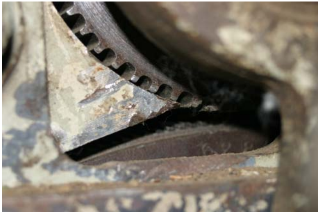
Figure 3 – Photo showing a high feed plate setting ( > 1/8^{\text{th}} inch) to saw (Lummus lint cleaner)
