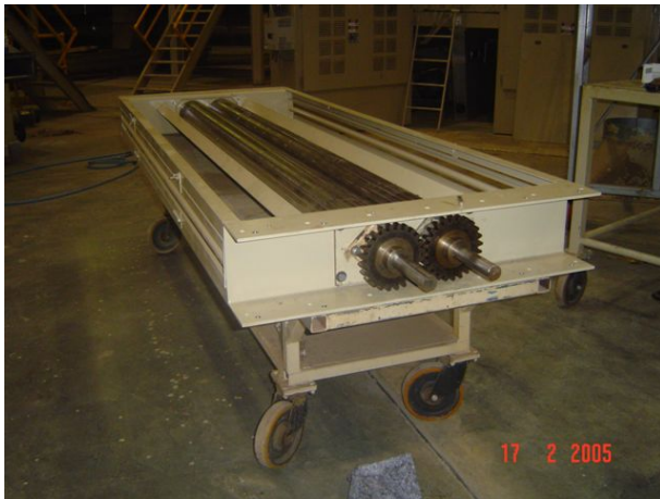
Figure 1 – Photo showing draft rollers and chassis fitted to the first lint cleaner on gin stand one in Gin 8 Auscott Narrabri. In the upgraded version the 150 mm rollers are replaced with 100 mm rollers and the chassis is reduced in thickness.
