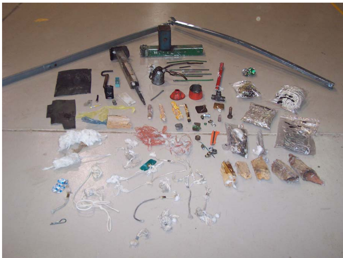
Figure 4 – Examples of contaminants collected from modules
