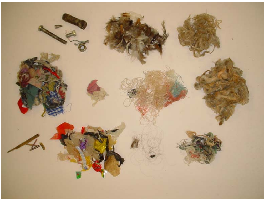
Figure 6 – Examples of contaminants collected from Australian lint bales
