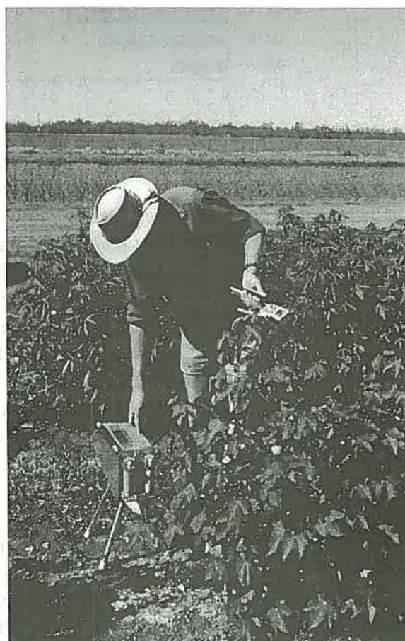
Measuring gas exchange characteristics of cotton with the Licor 6400
