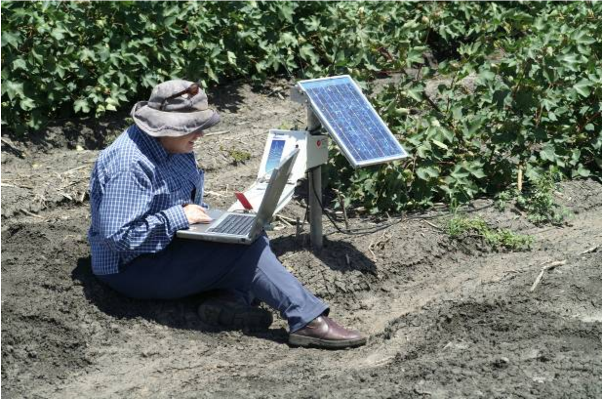
Photo 14 RWUE3 officer Jenelle Hare downloads EnviroSCAN data from cotton variety x irrigation demonstration at Dalby
