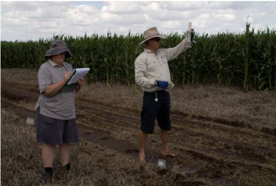
Photo 18 RWUE3 officer Jenelle Hare and local consultant Murray Boshammer, TAGS measuring catch can volumes during centre pivot evaluation
