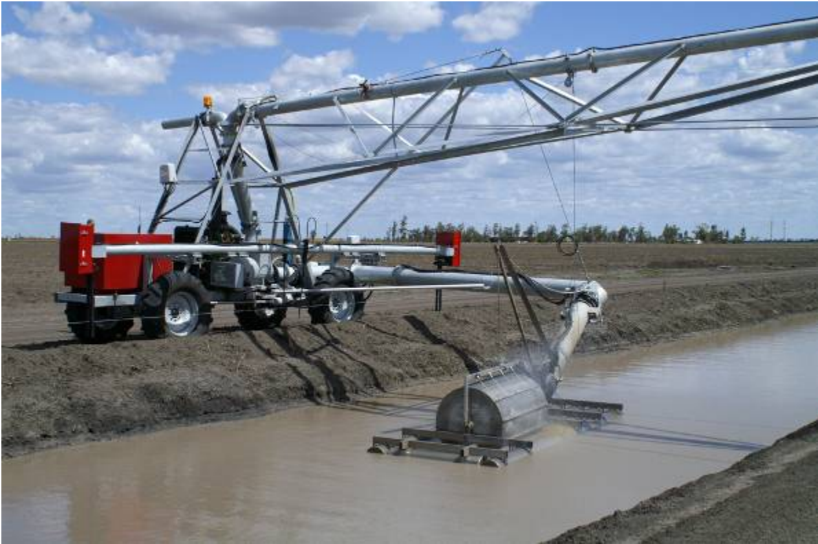
Photo 9 Lateral move installation on Darling Downs
