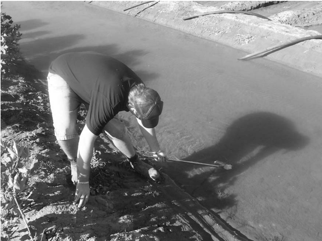
Figure 5 – Grab sampling technique
