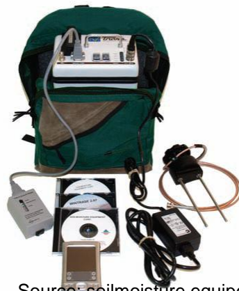
Figure 9: time domain reflectometry equipment
