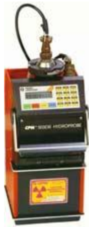
Figure 8: neutron probe with schematic of use
