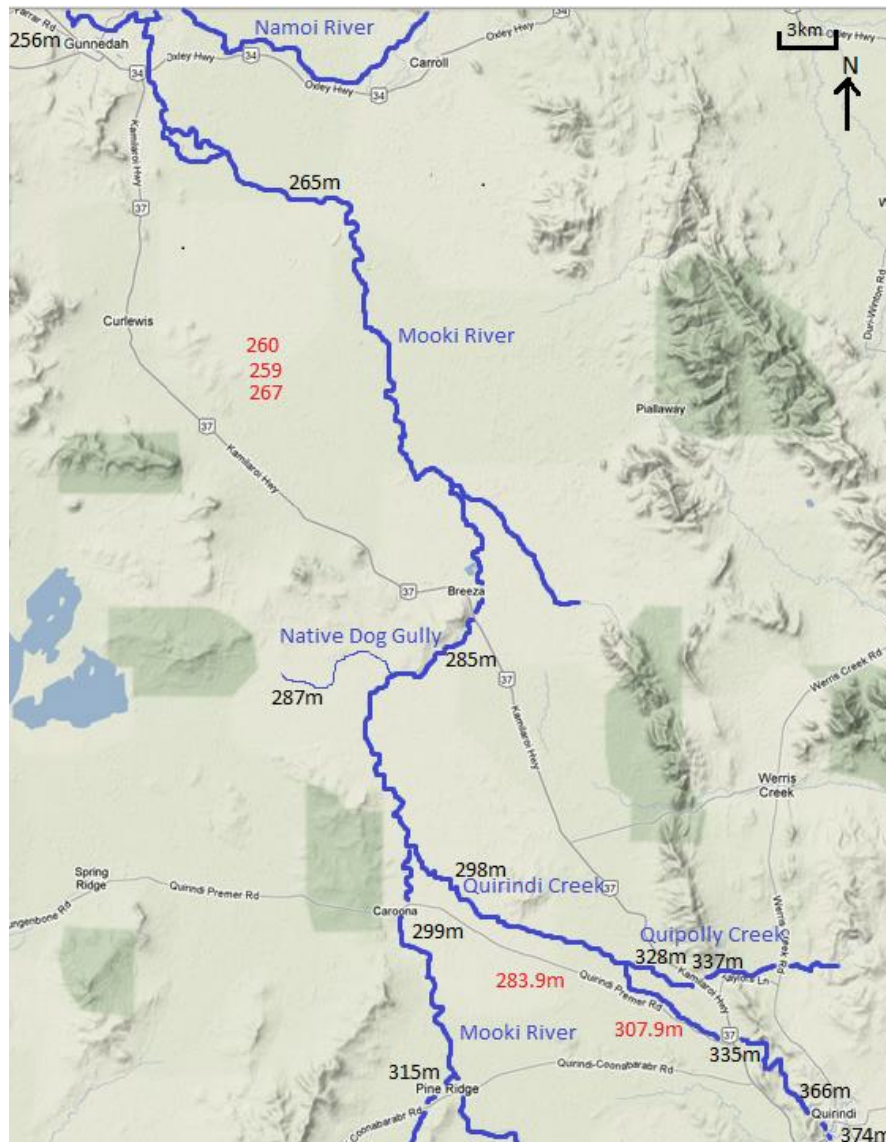
Figure 4.1.1: Mooki catchment stream and ground water levels (m AHD; surface water and groundwater reading are coloured black and red, respectively)
