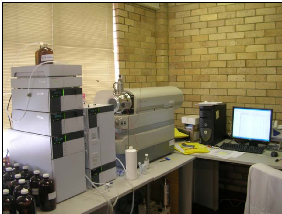
Fig. 4. Photograph of LC/MS/MS used to analyse samples for diuron.
