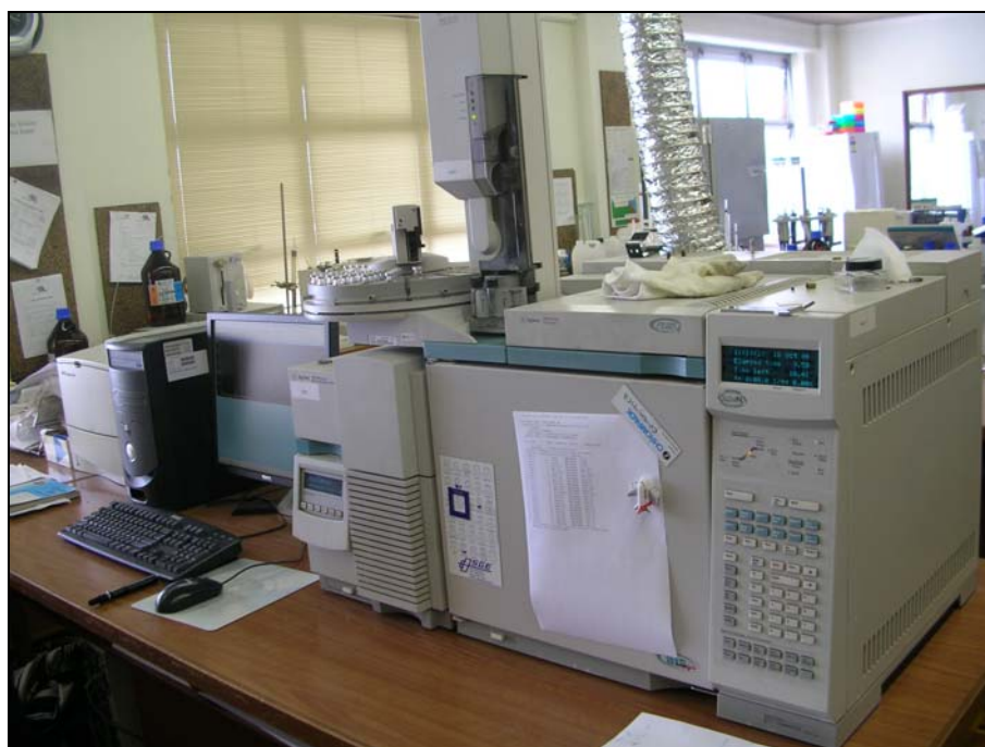
Fig. 5. Photograph of GC-MS used to analyse for endosulfan sulphate.
