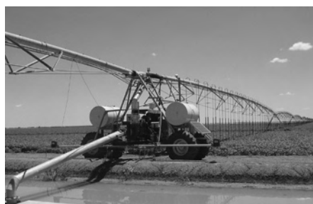
Auscott's lateral move system produced a yield increase of one bale per hectare
