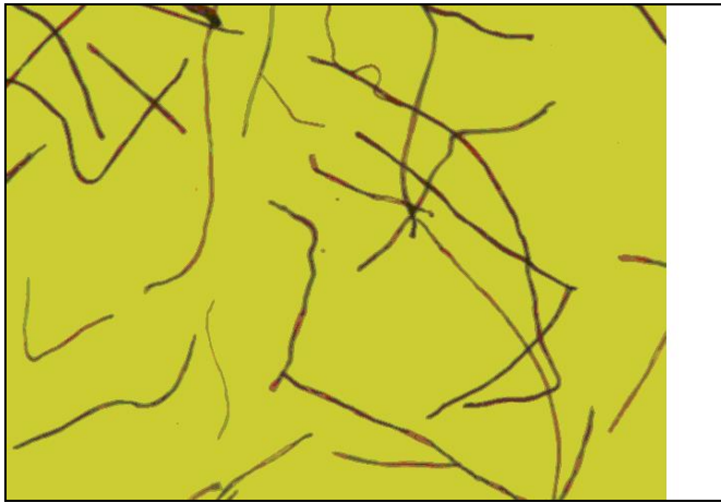
Figure 3 – Combined Cottonscope image showing mature (red) and immature (dark) fibre snippets (1 mm)
