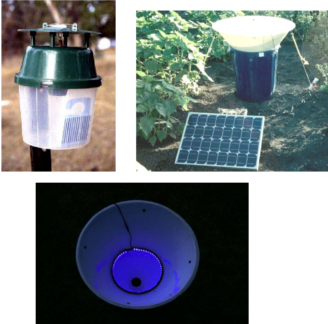
Fig. 5. (a) Unitrap pheromone trap with clear base to show killing agent (dichlorvos strip) - those used in this experiment had opaque green bases. (b) cone type light trap (c) light source for the trap, consisting of a ring of 60 waterproof UV LEDs.
