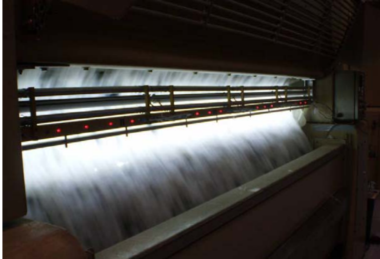
Figure 4-4 DAVS in position on gin stand apron.
