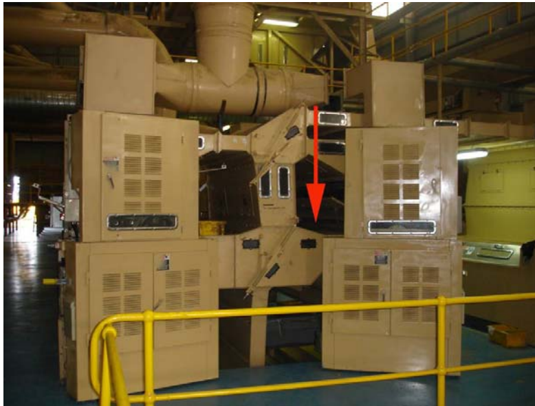
Figure 3-13 Lint sample collection availability after the 1 st and 2 nd lint cleaners.
