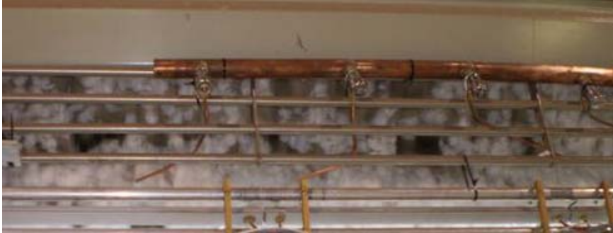
Figure 4-13 Air blowers in position for the manipulation of the seed cotton distribution prior to the gin stand.
