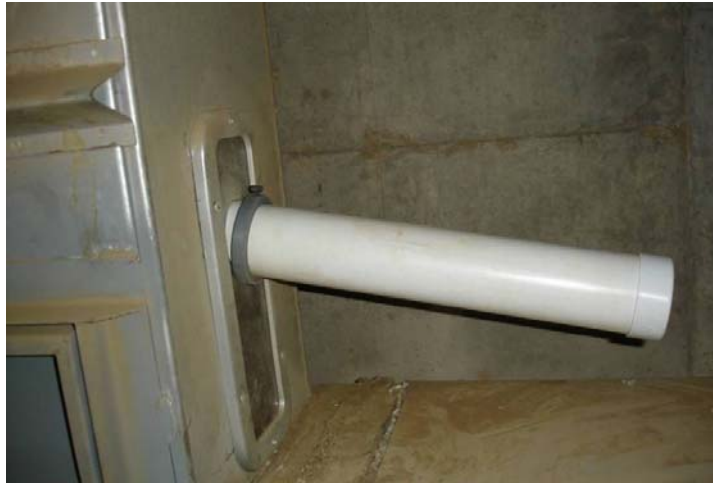
Figure 3-11 Seed tube fuzzy seed sample collection.
