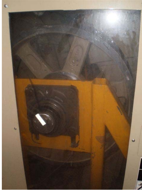
Figure 4-11 Saw shaft rigidity shaft and support in position
