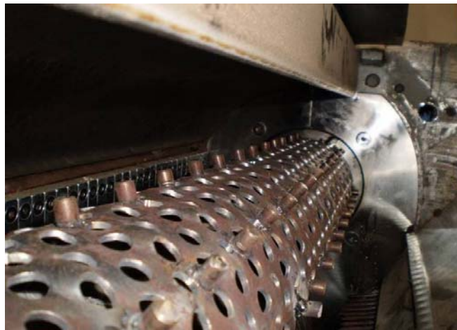
Figure 3-29 Modified seed tube.
