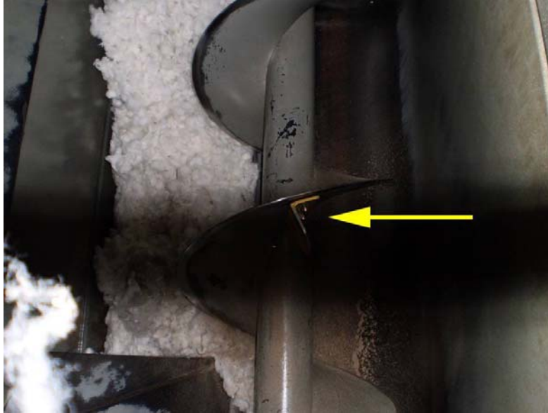
Figure 4-14 Conveyor distributor deflector mounted in position.
