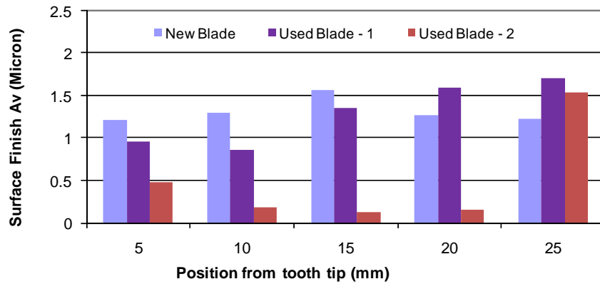
Figure 3-37 Saw blade surface finish (microns).
