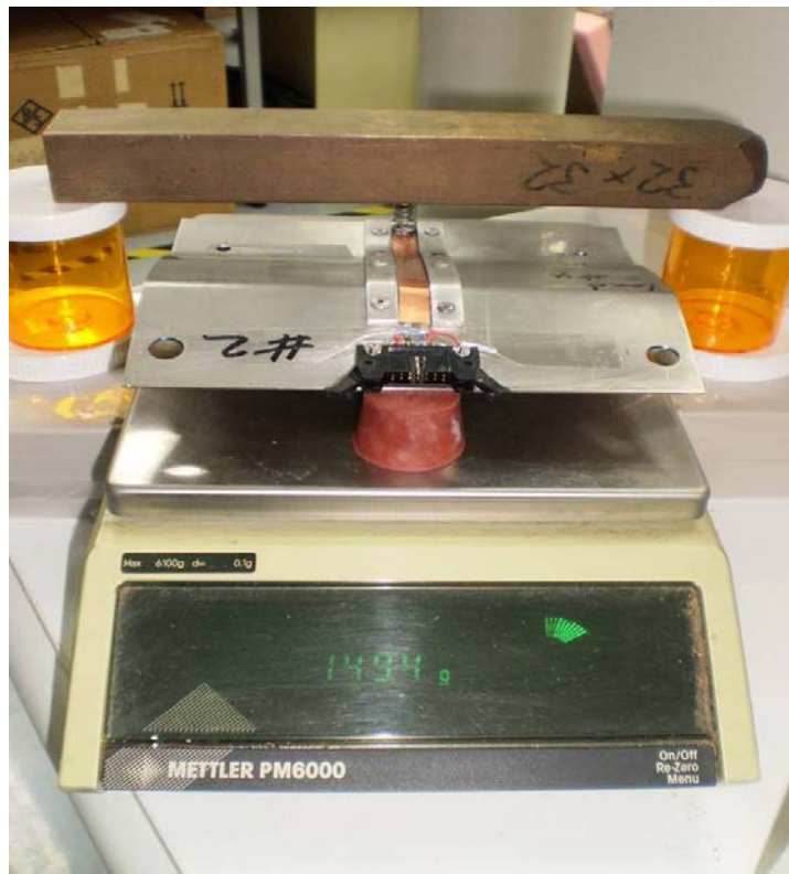
Figure 3-3 Seed roll force sensor calibration.
