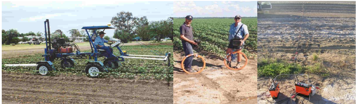
Figure 26. Assessing spatial distribution of root and vadose zone properties of sediments using a) Mobile Electromagnetic Sensing System (MESS), b) EM34 and c) direct electrical methods.
