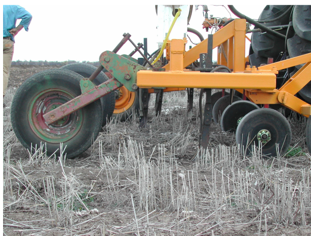
Figure 20. Modified anhydrous ammonia rig with coulter discs in front of gas knives
