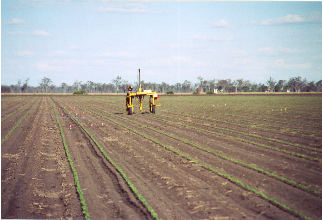
Installing neutron moisture access tubes using hydraulic soil sampler ('Moonbuggy') 2003-04
