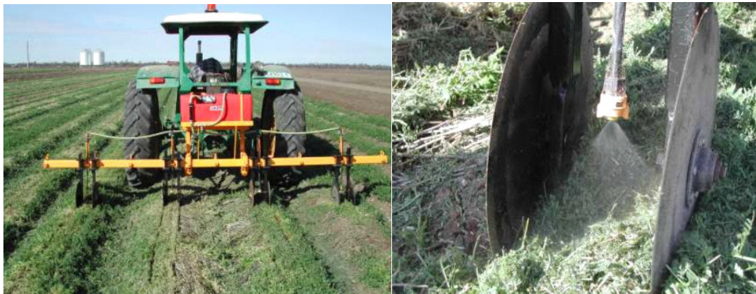
Figure 24. Simultaneously cutting off vetch runners and applying Sprayseed®
