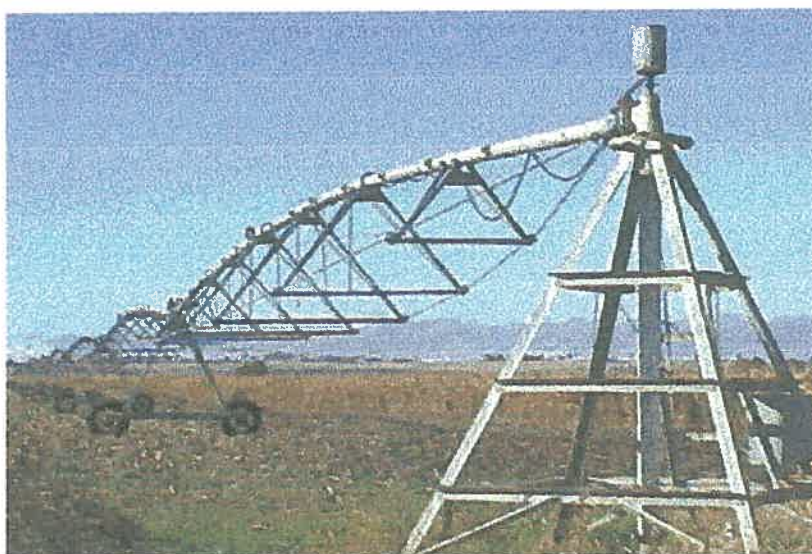
Figure 2.1: Centre pivot irrigation machine showing centre tower, spans, and wheel towers
