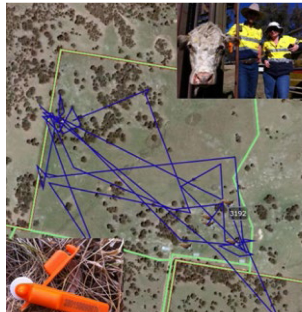
Figure 7: Wireless NLIS animal identification and tracking system to assist with herd management and breeding using Taggle ear tags.
