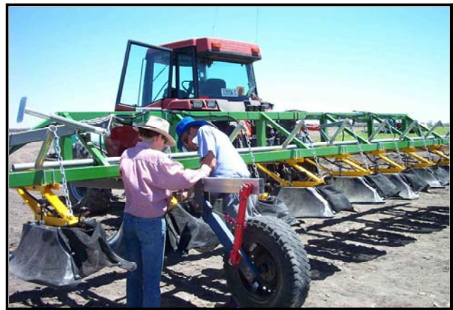
Plate 2 – The Polumbo shielded sprayer
