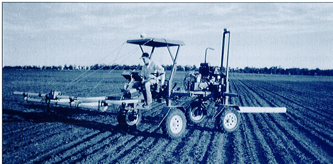
The Mobile Electromagnetic Sensing System, pictured, to assess soils salinity and related parameters on field, was designed by John Triantifilis during a CRDC-funded post-doctoral fellowship
