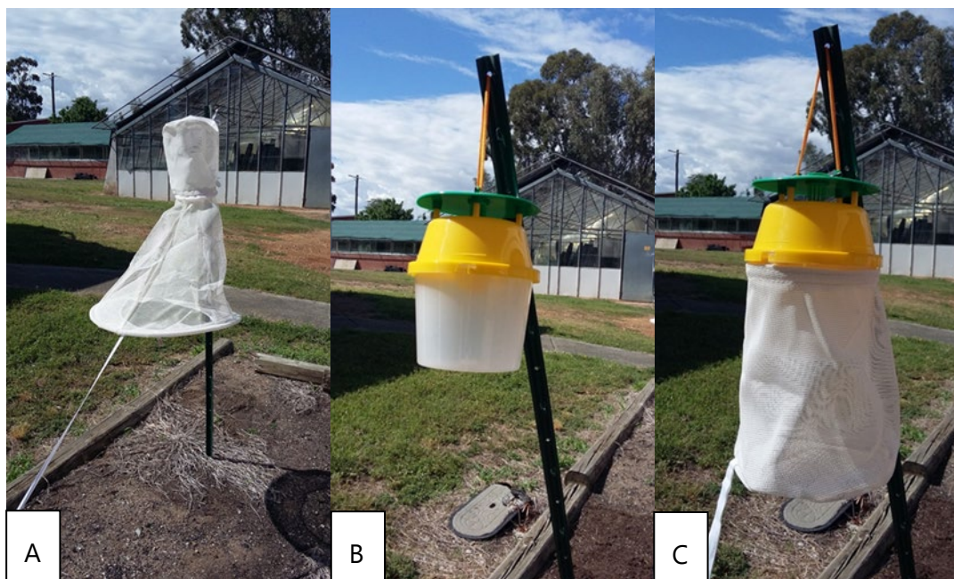
Figure 1.10.1 Pheromone trap designs: A Heliothis net trap; B standard unitrap; C modified unitrap with mesh trapping receptacle.
