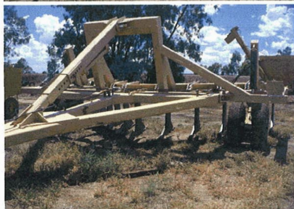
A trailing ripper set up for heavy cultivation of nutgrass after picking. Note the steel cable across the rippers (top photo) designed to cut the nutgrass roots during ripping.
