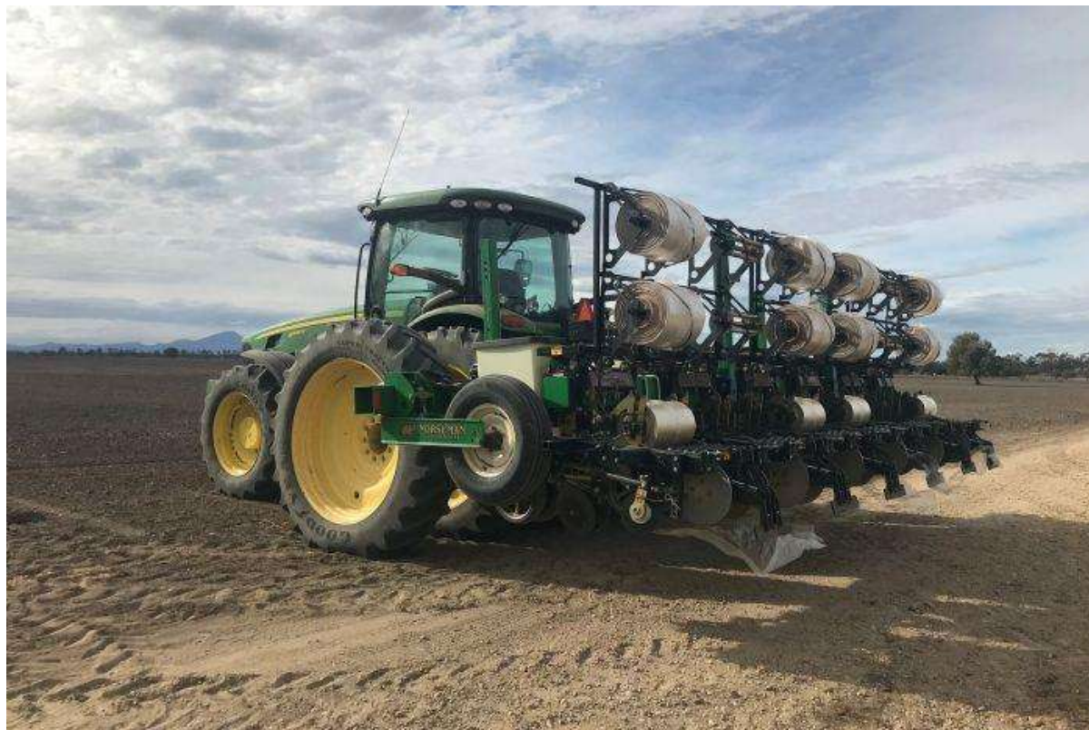
Figure 1. An example of the planting rig used to apply the biofilm at planting.
