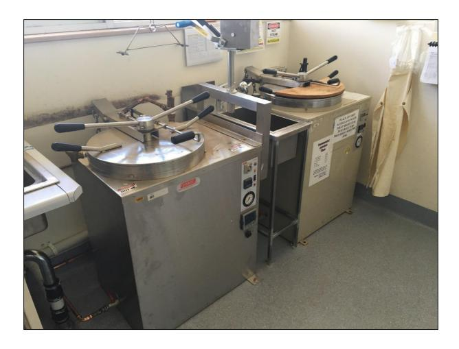
Figure 1: New Labec AA20 100 litre automatic autoclave is doubling ACRI laboratory capacity to process waste and sterilise laboratory equipment. (new unit on the left side)
