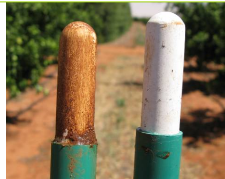
Figure 24 Ceramic cup sampling devices removed from soil in the Atwood navel orange irrigation/fertiliser management trial at Dareton
