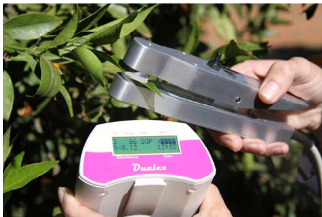
Figure 2 Hand held Dualex instrument for measuring leaf chlorophyll and phenolics
