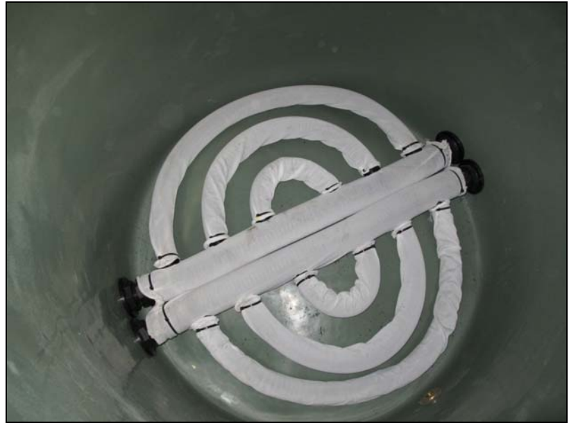
Figure 25 Drainage pipe and filter sock in bottom of lysimeter
