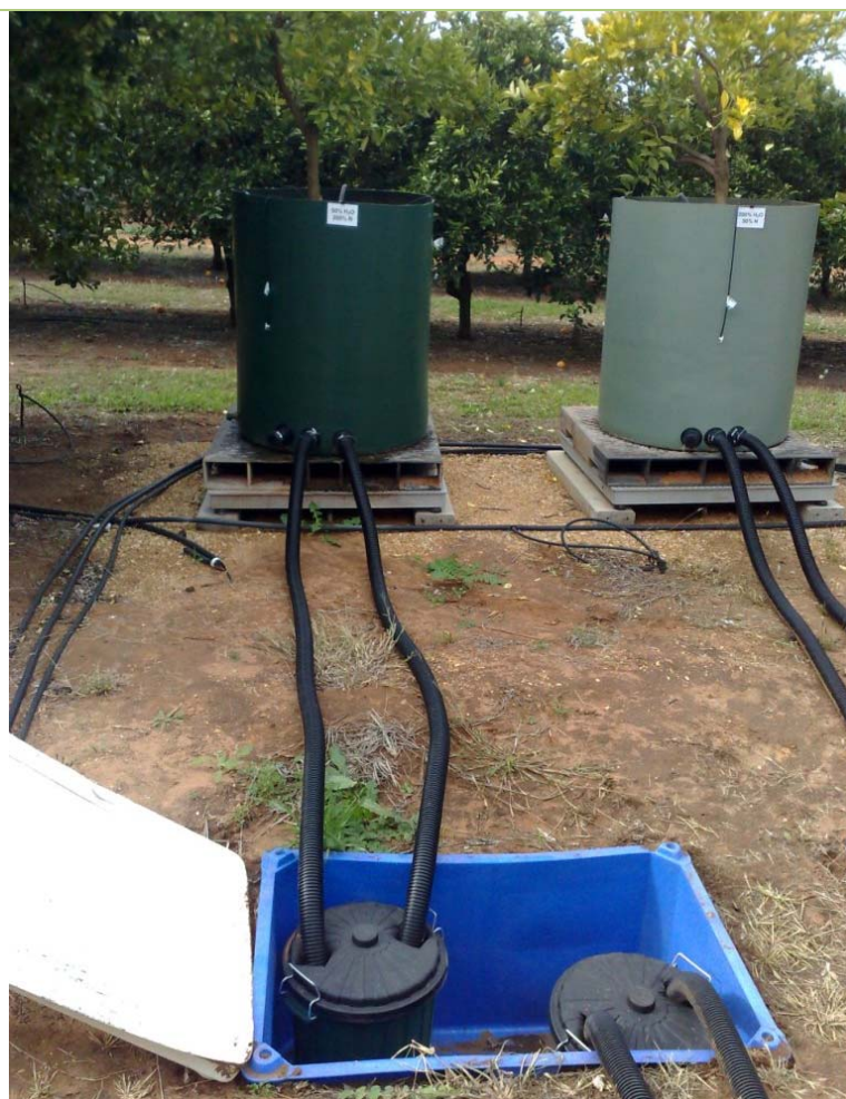
Figure 29 Lysimeter drainage collection apparatus
