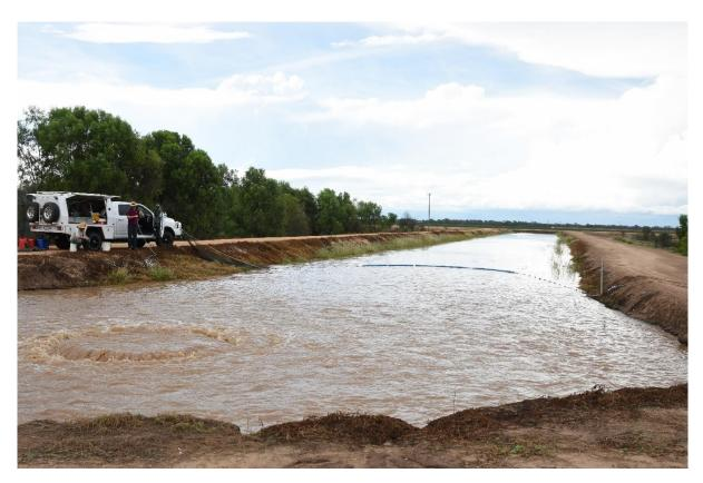
Figure 4: Outlet sampling net in place. Note the float line and extra floatation across the centre of the net.
