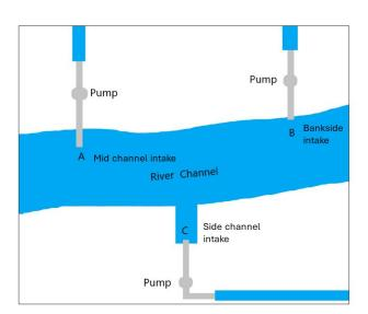
Bankside shallow intakes generally entrain far fewer native fish than other pump intake configurations. Entrainment rates of the other intake configurations vary between species, but overall, they have similar total impacts to each other.
