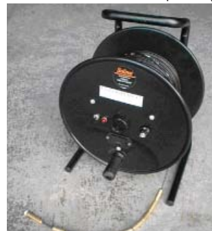
Figure 4 – Example of water level dipper and pocket sized salinity EC meter.
