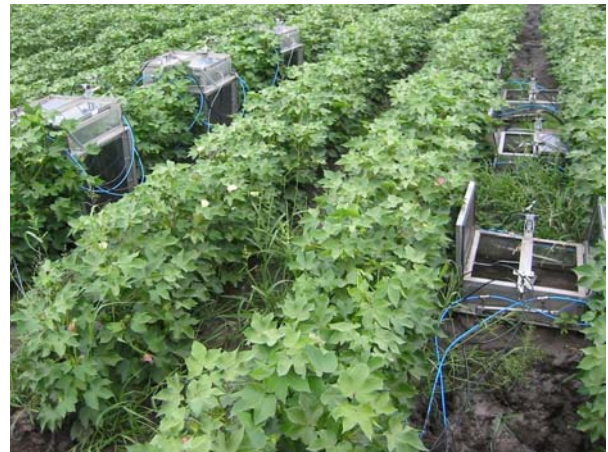
Above: Gas chambers as part of the farm trial measuring the greenhouse gases from a cotton crop east of Dalby, QLD.
