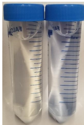
Figure 22. Water collected from the incubation bottles after aerobic biodegradation of cotton without finishes (left) and cotton dyed with Blue 19 (right). In this experiment, activated sludge from the Neuse River WWTP was used as inoculum at low concentration.
