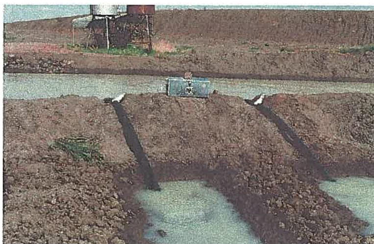
Figure 7: GLI tee-mount meter in irrigation siphons measuring water applied
