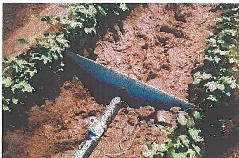
Figure 8: GLI tee-mount meter measuring tailwater from a furrow
