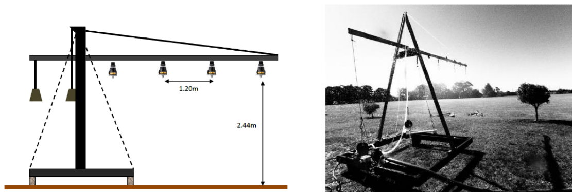
Figure 3: Mobile sprinkler rig constructed for the project
