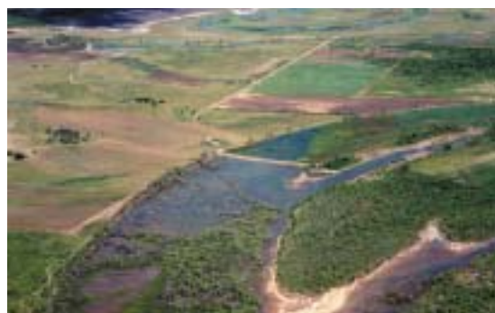
Photo 3: Saltwater intrusion bund wall on lower Kalamia, Burdekin Delta facilitates agricultural expansion to the margin of the delta soils.
