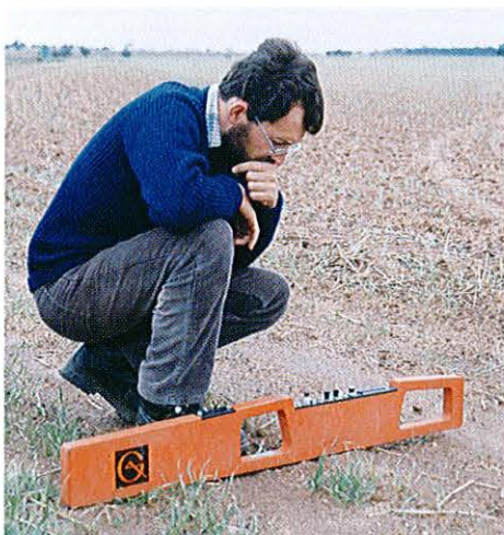
Photo 3.3 Measuring soil salinity with the EM38 (Photograph: Sue Wilkins).
