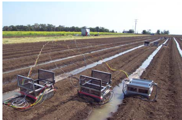
Figure 1. Chambers deployed in the spring of 2011. In the background is the trailer which houses the gas chromatograph and computer system used to measure the GHG concentrations in the chambers
