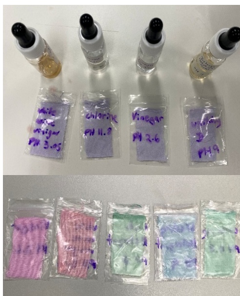
Figure 19. Colour-change capacity of Red Cabbage dye from varying pH values on cotton fabric.
