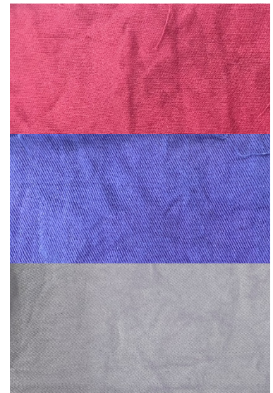
Figure 21. Close up photo of cotton fabric dyed with Hibiscus, Butterfly Pea flower and Red Cabbage.
