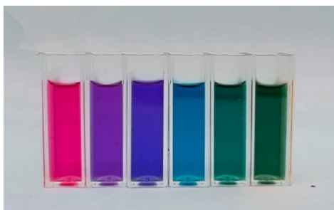
Figure 15. Butterfly pea flower extract colour changes after varying pH values were added.
