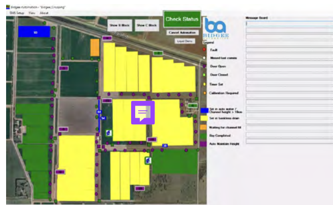
Figure 25: Colour coded dashboard enables easy visual checks of device status.
