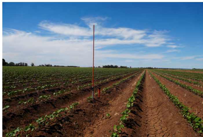
Figure 21: In field water height sensor.
