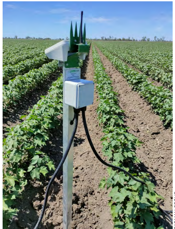
Figure 22: An in-field sensor provides data to inform irrigation decisions.
