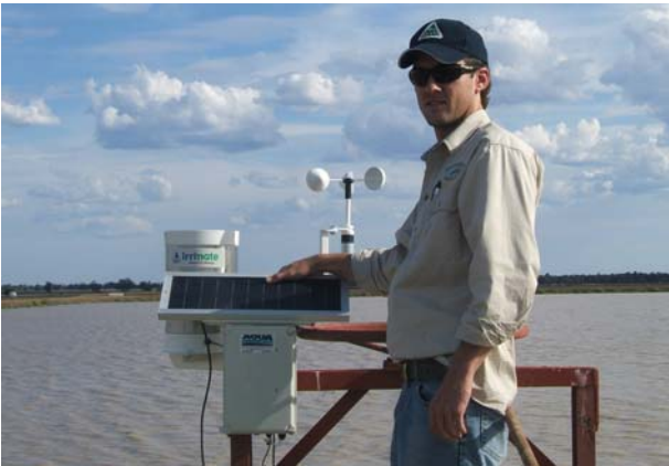
Plate 1 Wee Waa AIMS consultant Mitch Carter installing Irrimate storage evaporation meter
