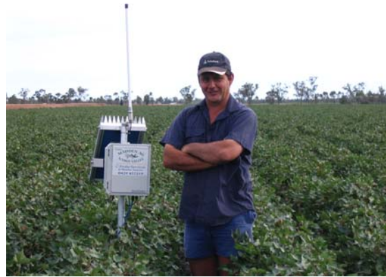
Plate 2 Cotton grower Paul Hawkins from 'Willawah' Wee Waa with soil moisture C-probe.
