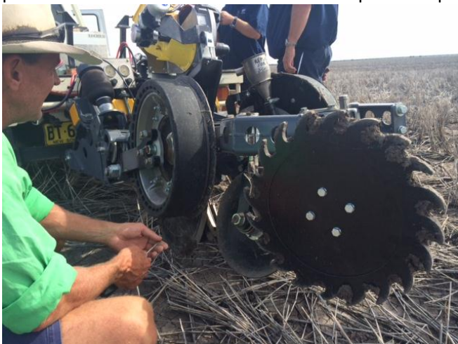
Note 2 airbags with trench disc and coulter on different pressure
