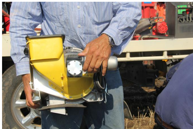
Electric powered precision seed boxes
