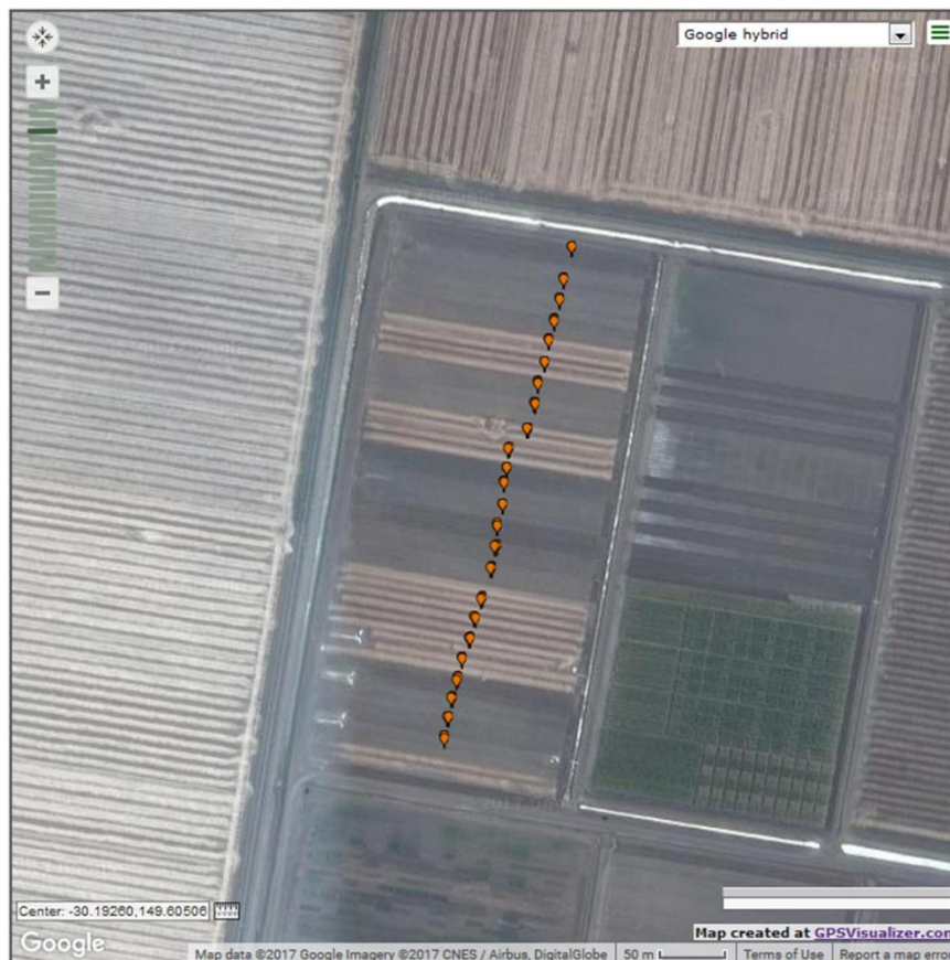
Figure 25 An overlay of the RTK GPS positions of the cone penetrometry sites take in May 2017. Similar results were plotted with each sampling. The step in the sampling (toward the top of the image) was due to the lysimeter, which was located in plot 16. There are actually three pins at each point (two furrow and one hill), but the field boundaries are lost with further magnification.
