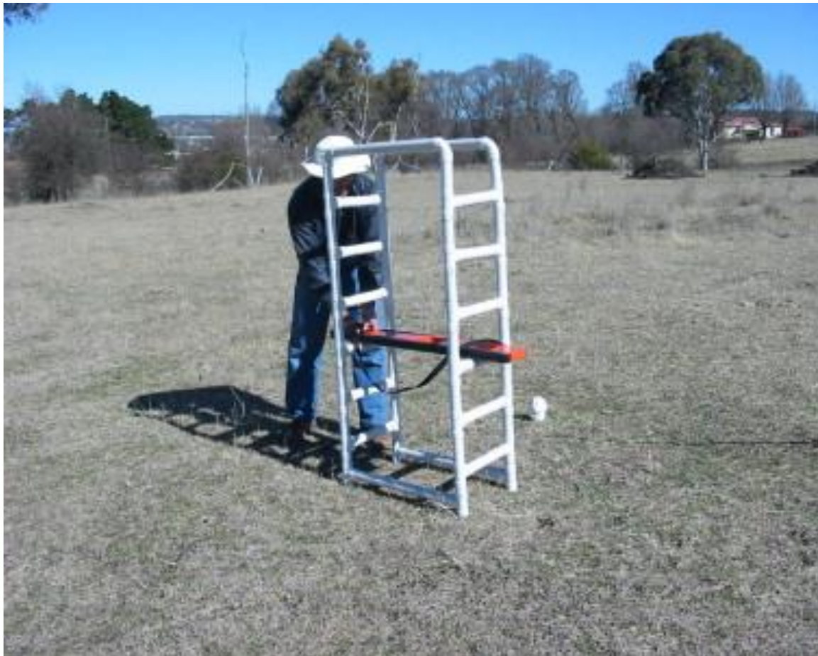
Figure 2.21 Polymer ladder device for multi-height EM38 measurements (after Hossain et al., 2010)
