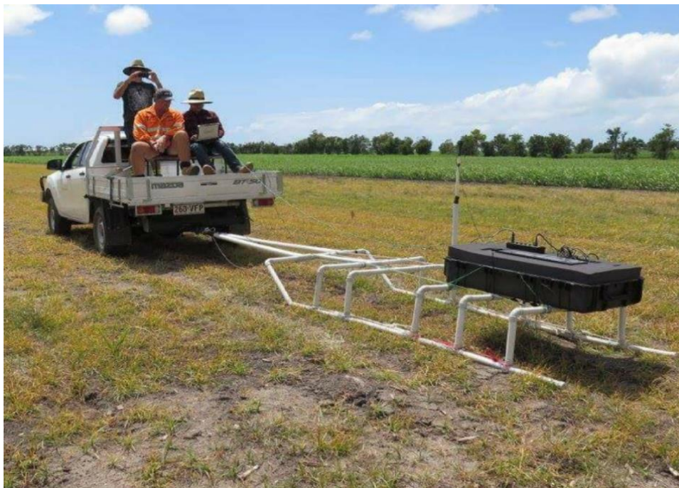
Figure 2.31 Proximal RS-700 \gamma -ray spectrometer (Radiation Solution INC, Ontario, Canada) being towed on a PVC sled.
