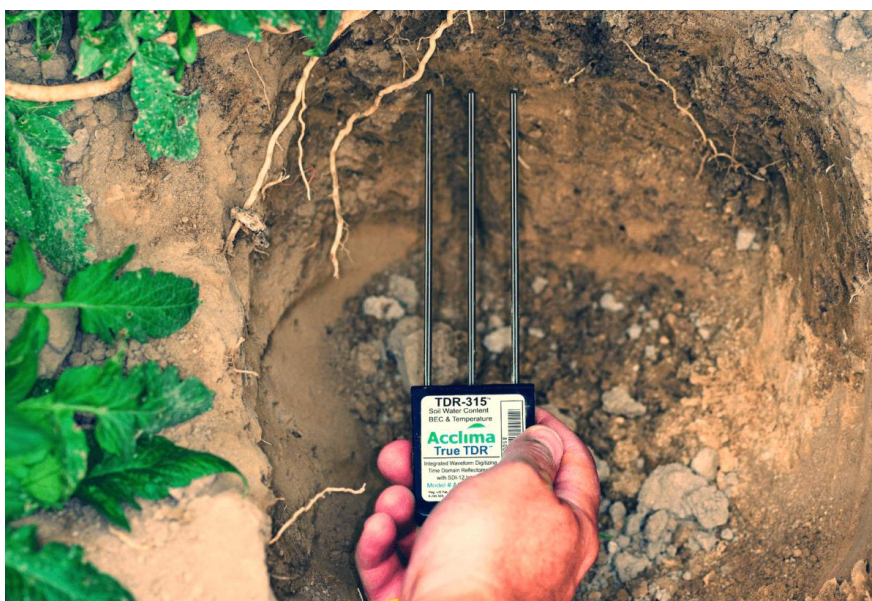
Figure 2.2 Acclima TDR-315 (Meridian, Idaho USA) moisture sensor (access from https://soilsensor.com/articles/time-domain-reflectometry-tdr/ ).
