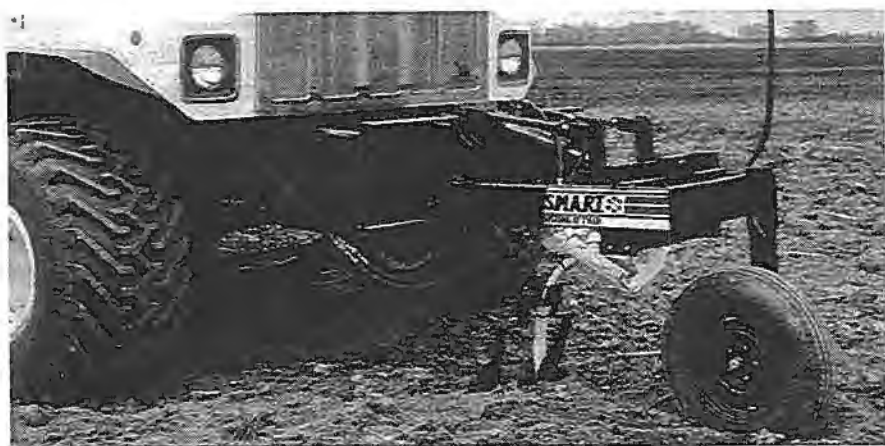
Figure 18. Mounting system for the tines
