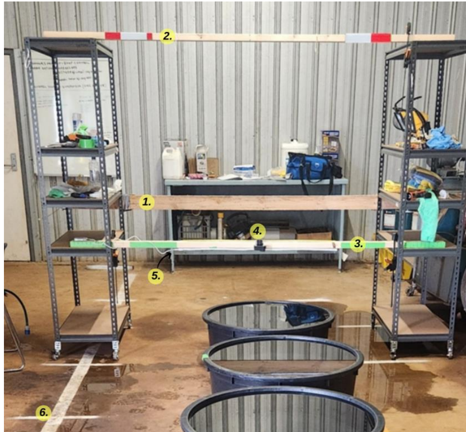
Figure 2.2.2 Annotated apparatus setup. 1. Fixed timber beam 2. Top beam 3. Mounting beam 4. GoPro 5. LED Light Strip 6. Floor spacing markers.
