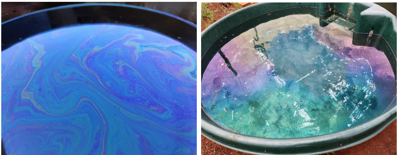
Figure 1.4.2 PDMS Film in bucket (left) and trough (right) trial showing thin film interference and reflective properties. (Source Sarah Seton 2023)
