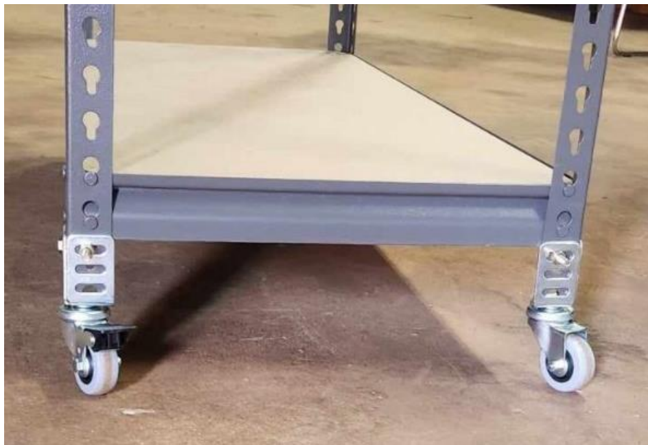
Figure 2.2.1 Assembly of data collection apparatus, demonstrating locking castors on the outer edge.
