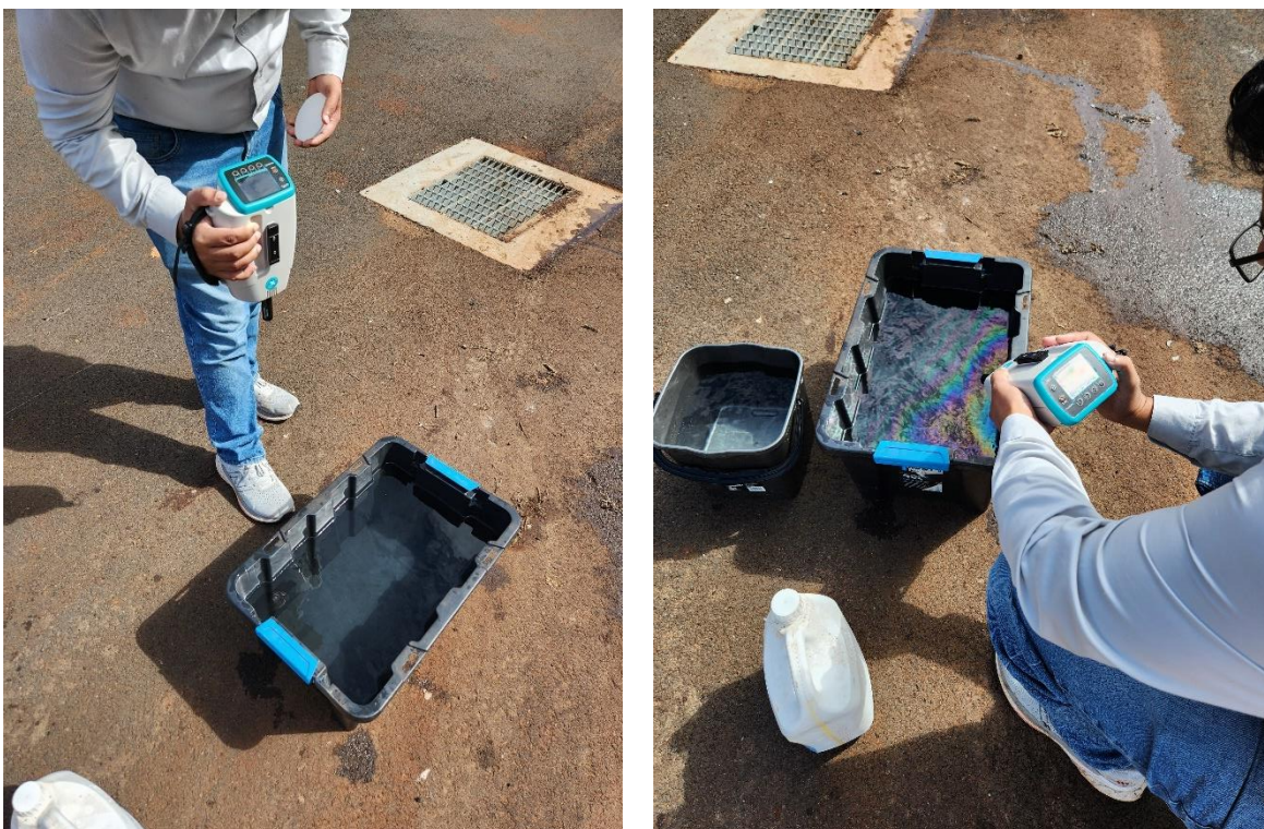
Figure 2.2.4 Preliminary experiment using ASD HandHeld2 VNIR Spectroradiometer on multimolecular film, located outside of P6 UniSQ Toowoomba Campus. (Photographs: Sarah Seton)
