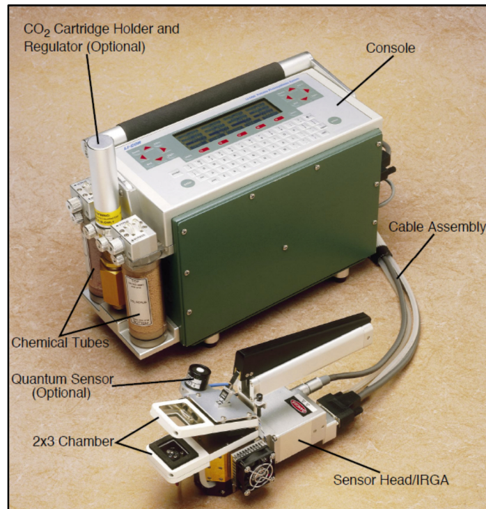
Figure 4-10. Main parts of the Li-6400 portable photosynthesis system. Source: (LiCOR, 1999)
