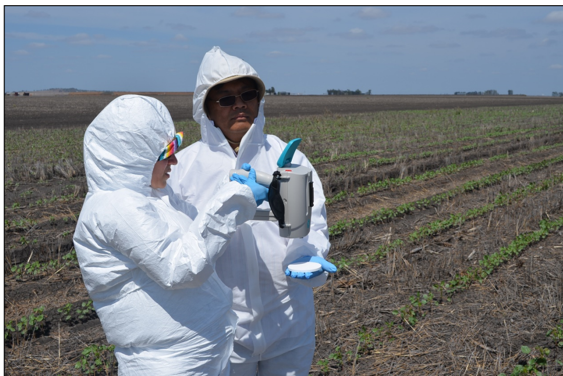
Figure 4-8. Calibration and optimisation procedure with a Spectralon ® white reference panel.
