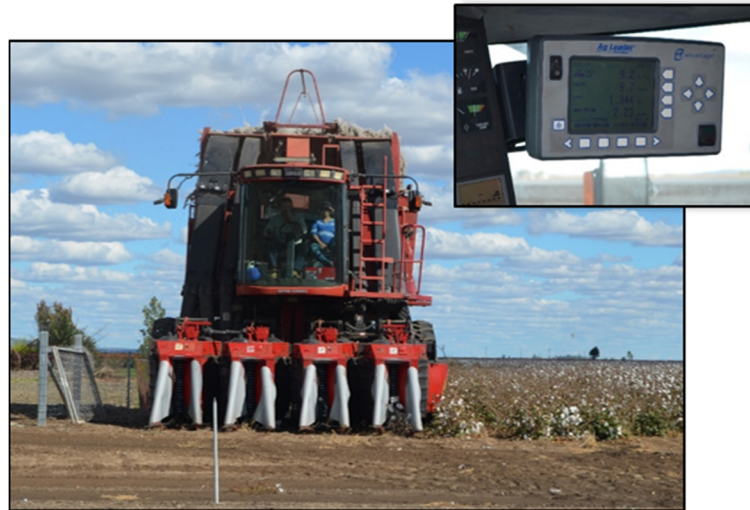
Figure 5-3. Picker and yield monitor implemented in this study.
