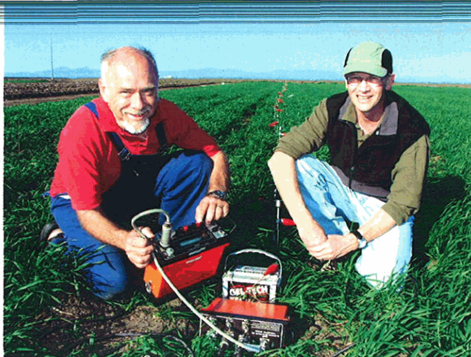
Figure 1: ABEM Terrameter SAS 4000. The multi-electrode resistivity imaging cable connected to the steel electrodes extends away from the meter through the centre of the background. (Image courtesy of Guy Roth and Anthony Nadelko)
