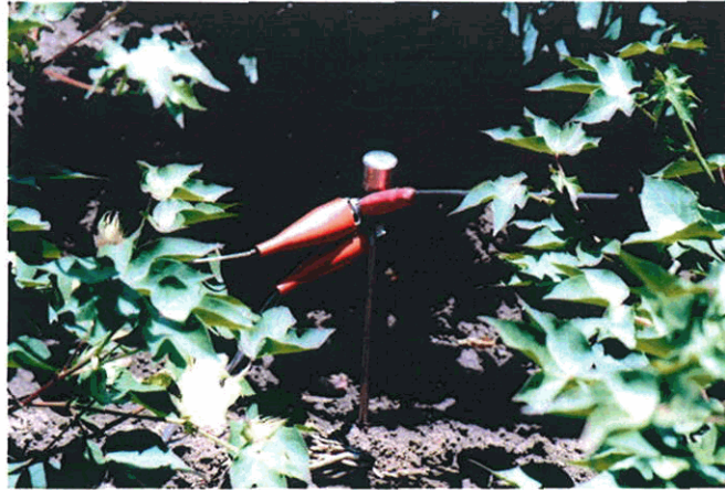
Figure 2: A close-up of the multi-electrode resistivity cable connected to a steel electrode.
